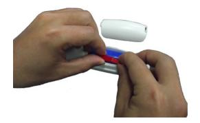
Step 3 : Directly insert the Light Guide into the curing light handpiece. Verify it has been completely inserted into handpiece. Light guide may be rotated to achieve best angle on tooth structure.
